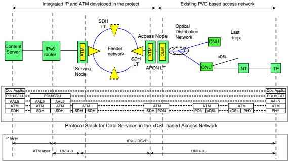
Signalling and control flows in the xDSL based Access Network
