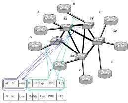
configure because a way to assign frames to tree instances is needed. In the case of MSTP, this means that the mapping of VLANs to tree instances (MSTIs) has to be configured manually at each bridge, resulting in a complex and error-prone process.
