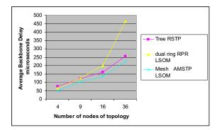
Fig. 8. Average backbone delay
