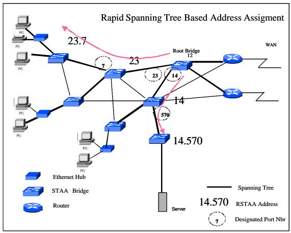
Fig.2 RSTAA addresses assignment principle
