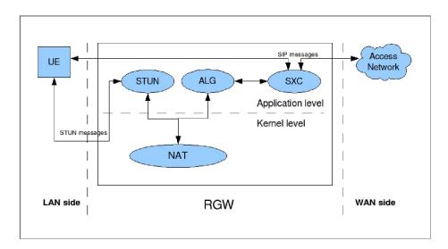
Fig. 3. ALG block in a NGN RGW
