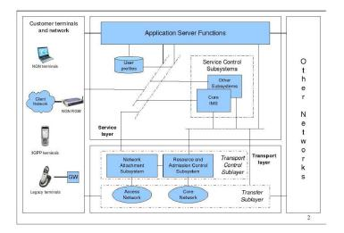
Fig. 1. Functional architecture of TISPAN NGN, release 1.
