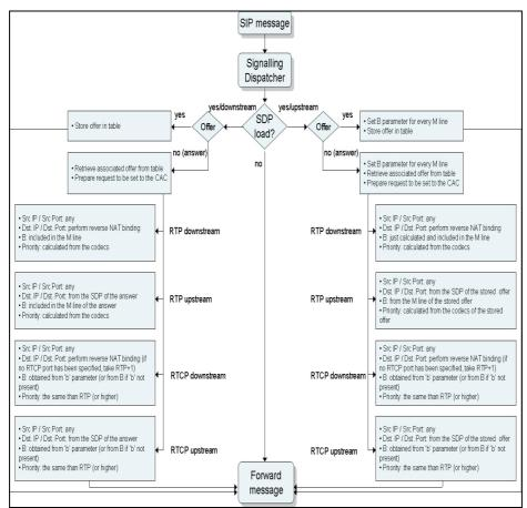
Fig. 5. Automatic configuration
