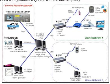
Fig. 6. Network trial testbed
