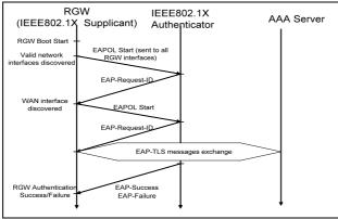
Fig. 3. RGW interface discovery and authentication.
