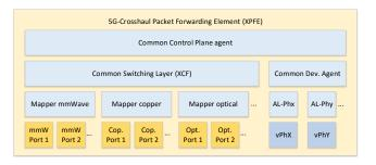
Fig. 3. 5G-Crosshaul Packet Forwarding Element
