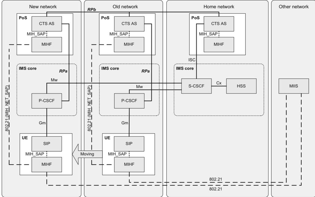
Figure 11: Architecture of the Context Transfer Service
