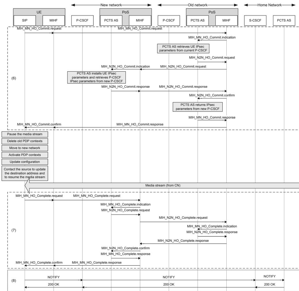
Figure 15: PCTS Phase 3 - Handover completion
