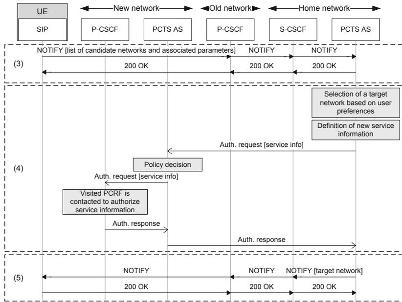
Figure 14: PCTS Phase 2 - Network selection procedure
