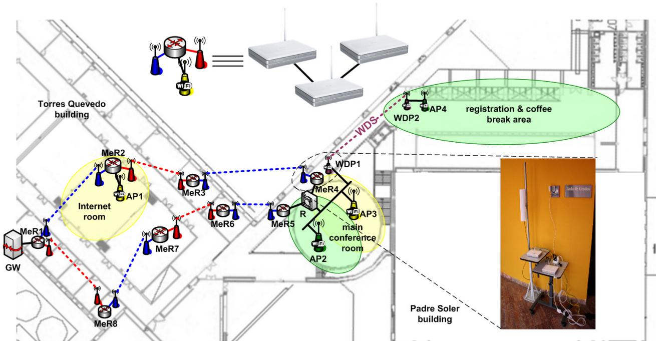
Figure 1. Mesh deployment
