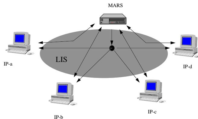
**Figure 3: Communication between MARS and LIS clients**
