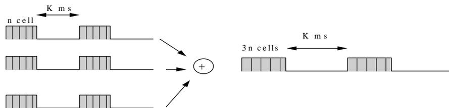
**Figure 6: Peak addition requires shaping on output**
