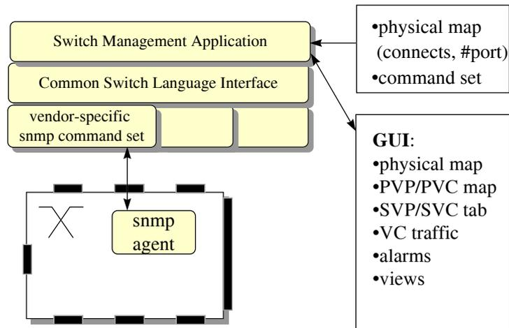
**Figure 7** ATM LAN Configuration and Management Application Architecture
