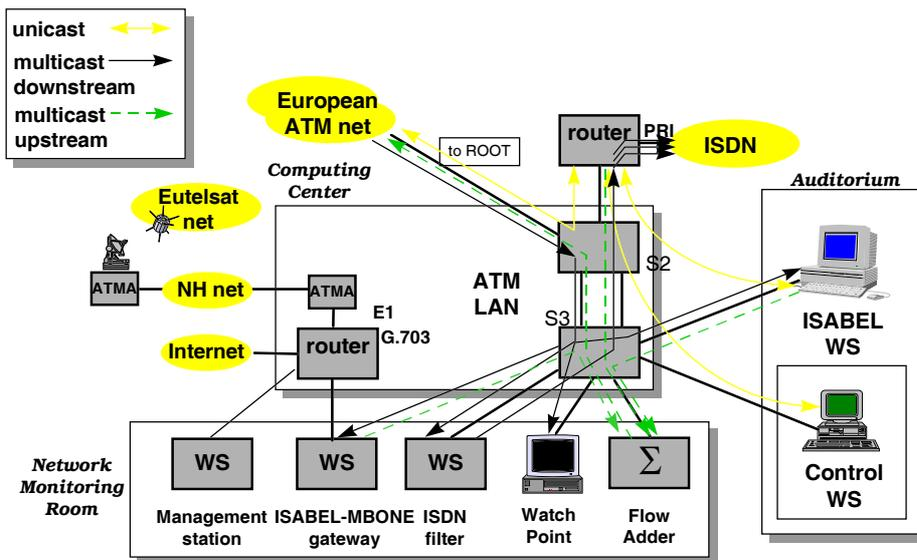
Figure 3 A complex Network Node with gateways to several networks
