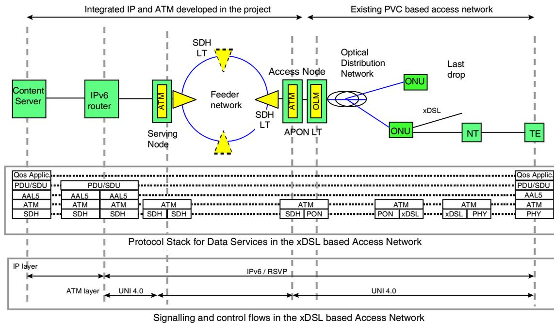
Fig. 1. Architecture of PON / VDSL based access network
