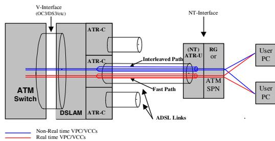
Figure 3. A reference model for an ATM-based ADSL system
