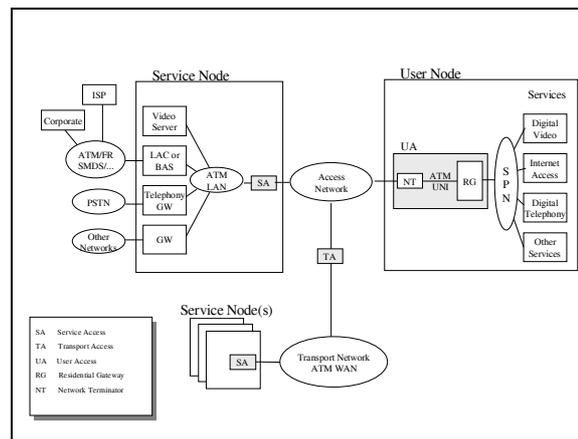
Figure 2. ATM-based integration of access and transport networks.
