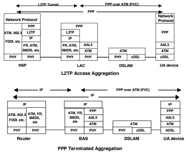
Figure 5. Comparison of L2TP Access and PPP Terminated Aggregation.
