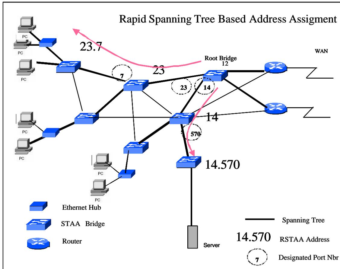
**Fig.2** RSTAA addresses assignment principle
