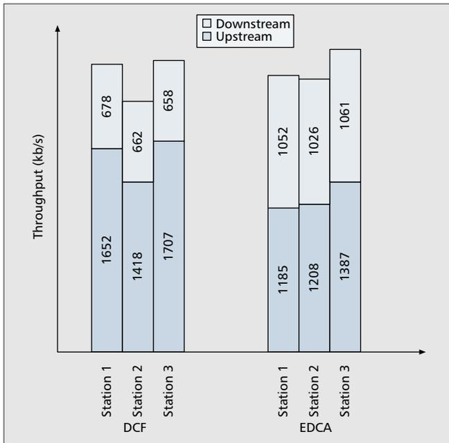
■ Figure 2. Symmetric traffic allocation with UDP traffic.
