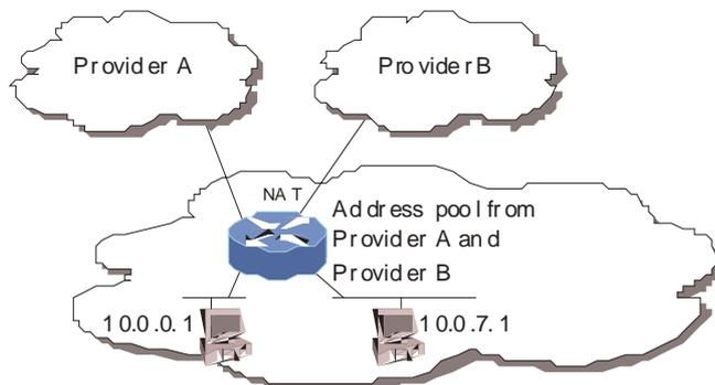
Figure 2: NAT-based Multihoming in IPv4 Networks.
