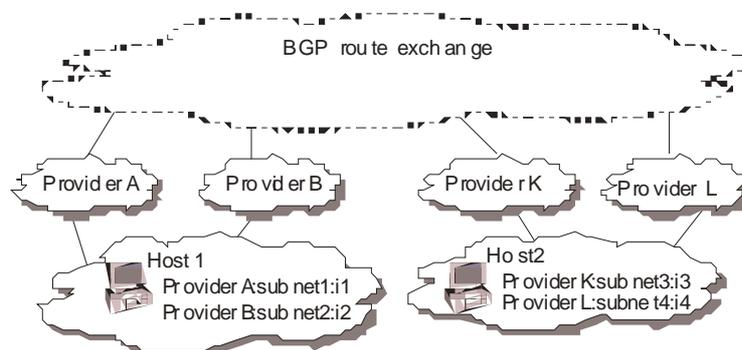
Figure 3: Multiaddressing-based Multihomed in IPv6.
