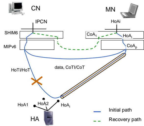
Figure 5. Response to a failure in RO mode
