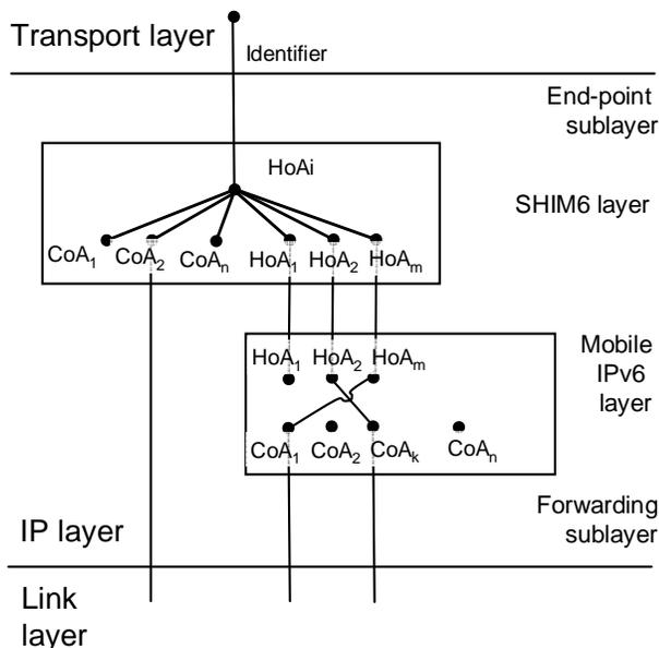
Figure 4. Mobile node multihoming architecture
