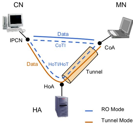
Figure 1. MIPv6 operation
