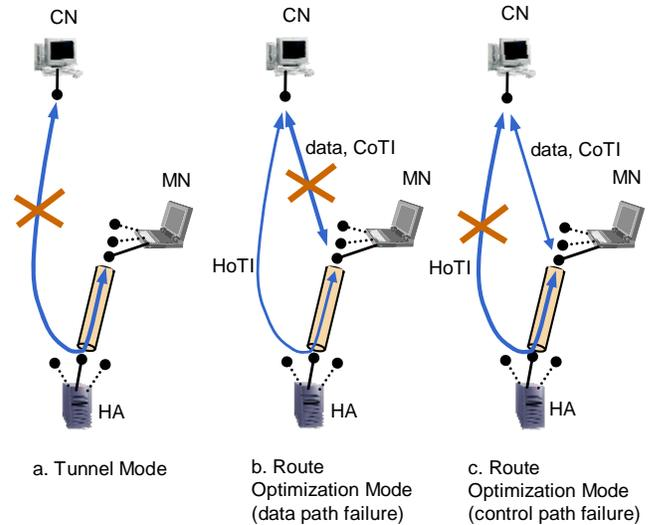
Figure 3. Failure scenarios for a multihomed MN
