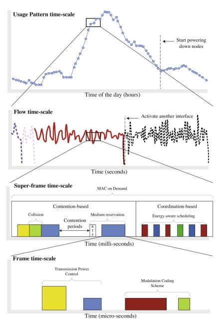
Fig. 1. Operational time-scales of the energy-saving algorithms.
