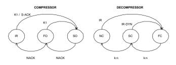
Figure 3: Compressor and decompressor state-machine.
