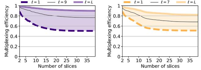
Fig. 16. Efficiency of slice multiplexing as a function of the number of slices  $k+1$  (on the x axis), when the  $k$  services with the highest traffic load have a dedicated slice and the remaining services are aggregated into a common slice. Thick dashed and solid lines denote the extreme network levels  $\ell = 1$  and  $\ell = L$ , while the thin solid line follows an intermediate network level. Left: large metropolis. Right: medium-sized city.
