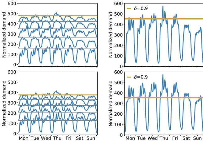
Fig. 5. Examples of multiplexing efficiency, when  $\delta = 0.9$  expressed in time slots (top) and traffic volume (bottom).
