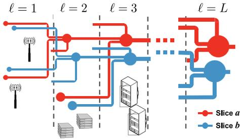
Fig. 2. Mobile network architecture. Nodes map to different equipment depending on the level  $\ell$ , and form a hierarchy. The mobile traffic in each slice (e.g.,  $a$  or  $b$ ) is increasingly aggregated as it flows from radio access to network core.
