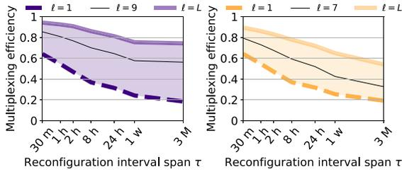
Fig. 14. Efficiency of slice multiplexing versus the resource reconfiguration periodicity  $\tau$ . Thick dashed and solid lines denote the extreme network levels  $\ell = 1$  and  $\ell = L$ , the thin solid line follows an intermediate network level. Left: large metropolis. Right: medium-sized city.
