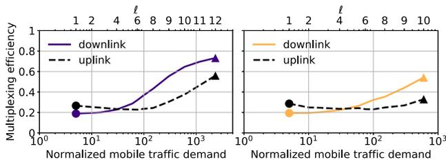
Fig. 11. Efficiency of slice multiplexing, in the same settings of Figure 10, separating downlink and uplink. Left: large metropolis. Right: medium-sized city.
