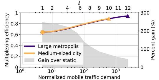
Fig. 13. Efficiency of slice multiplexing (left y axis) and percent gain over static assignment (right y axis) versus the normalized mobile traffic served by one node (bottom x axis) at level  $\ell$  (top x axis) in the two reference urban scenarios. Results are for a dynamic resource assignment where re-configurations occur with periodicity  $\tau = 30$  minutes, under slice specification  $z$  with  $\delta = 1$  and  $\pi = 0$ .
