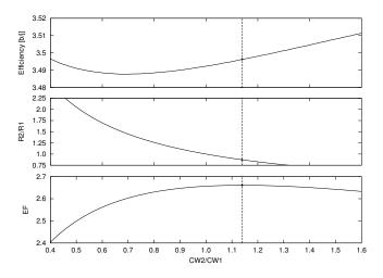
Fig. 1. Total efficiency, throughput ratio and EF performance of a WLAN with two stations for different CW configurations.
