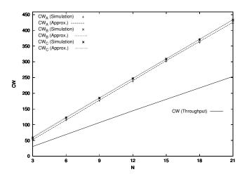
Fig. 3. Optimal CW configuration according to the accurate and approximate energy consumption models for a heterogeneous WLAN with interfaces A, B and C.
