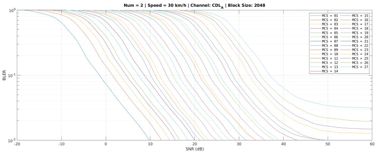
Figure 16. BLER for numerology 2, speed 30 km/h, CDL<sub>A</sub> channel model, and block size 2048.
