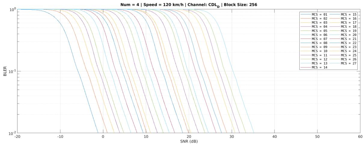
**Figure 17. BLER for numerology 4, speed 120 km/h, CDL<sub>D</sub> channel model, and block size 256.**
