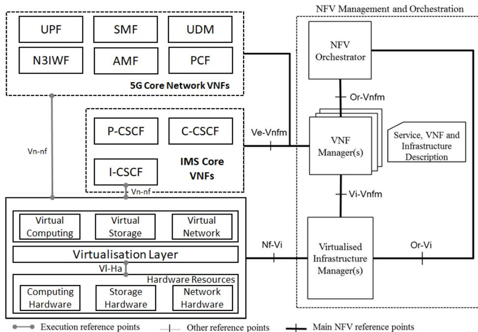
Figure 7. ETSI Network Function Virtualisation Architecture
