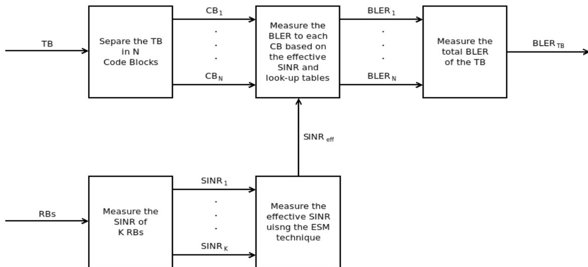
Figure 11. NS-3 implementation of the L2S interface providing the  $SINR_{eff}$  and BLER.
