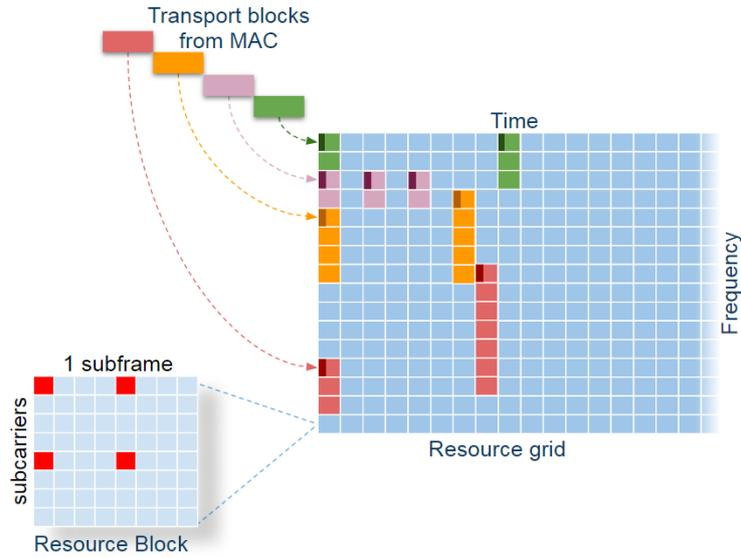
**Figure 1. Transport block allocation to the resource grid.**
