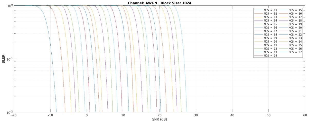
Figure 15. BLER curves for different MCSs. AWGN channel model and block size 1024.
