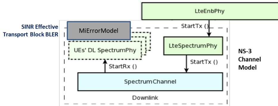
Figure 12. NS-3 Channel Model implementation and downlink transmission/reception.
