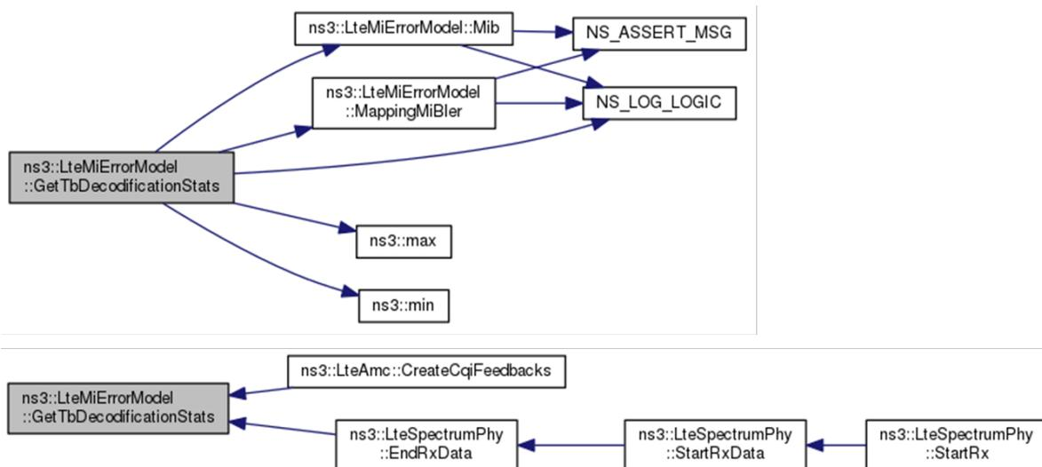
Figure 13. NS-3 Channel Model classes `LteSpectrumPhy` and `LteMiErrorModel` responsible channel model data transmission and reception and error model.
