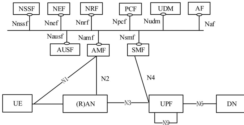
**Figure 6. Non-roaming 5G Core Network architecture using service-based model.**
