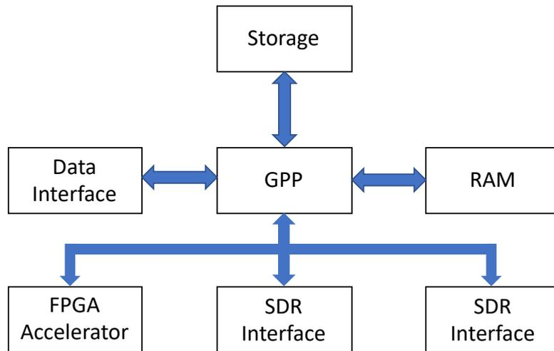
**Figure 23. Architecture of the SDR-based platform.**
