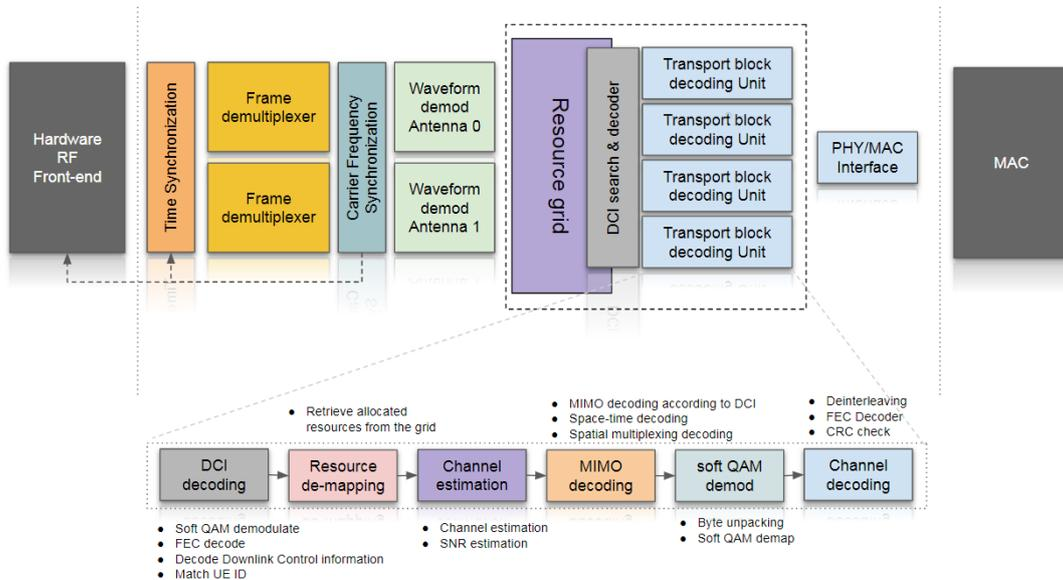
**Figure 3. Block diagram of the UE Receiver at the downlink.**
