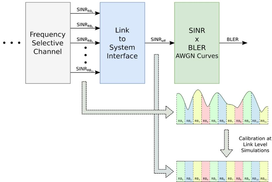
**Figure 8. Link-to-system (L2S) interface modeling.**
