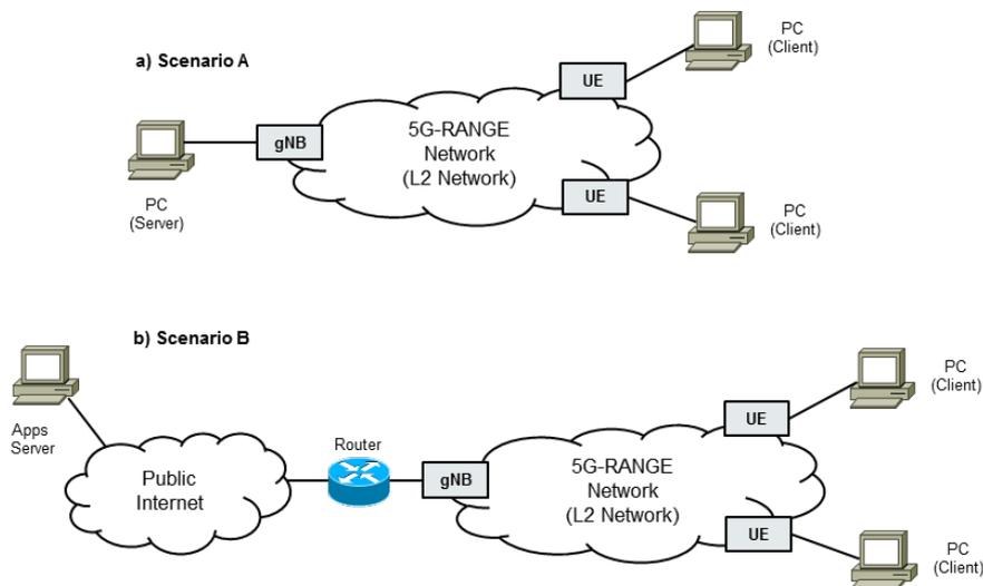
Figure 5. Options for PoC deployment for the 5G-RANGE network interconnections.
