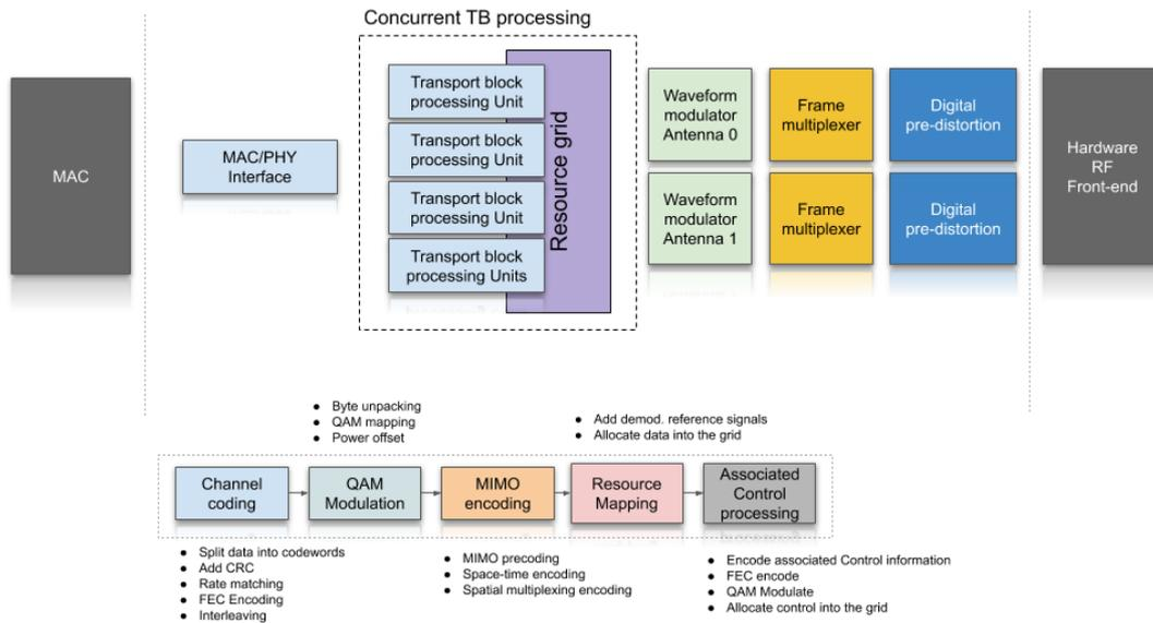
**Figure 2. Block diagram of the BS transmitter at the downlink.**
