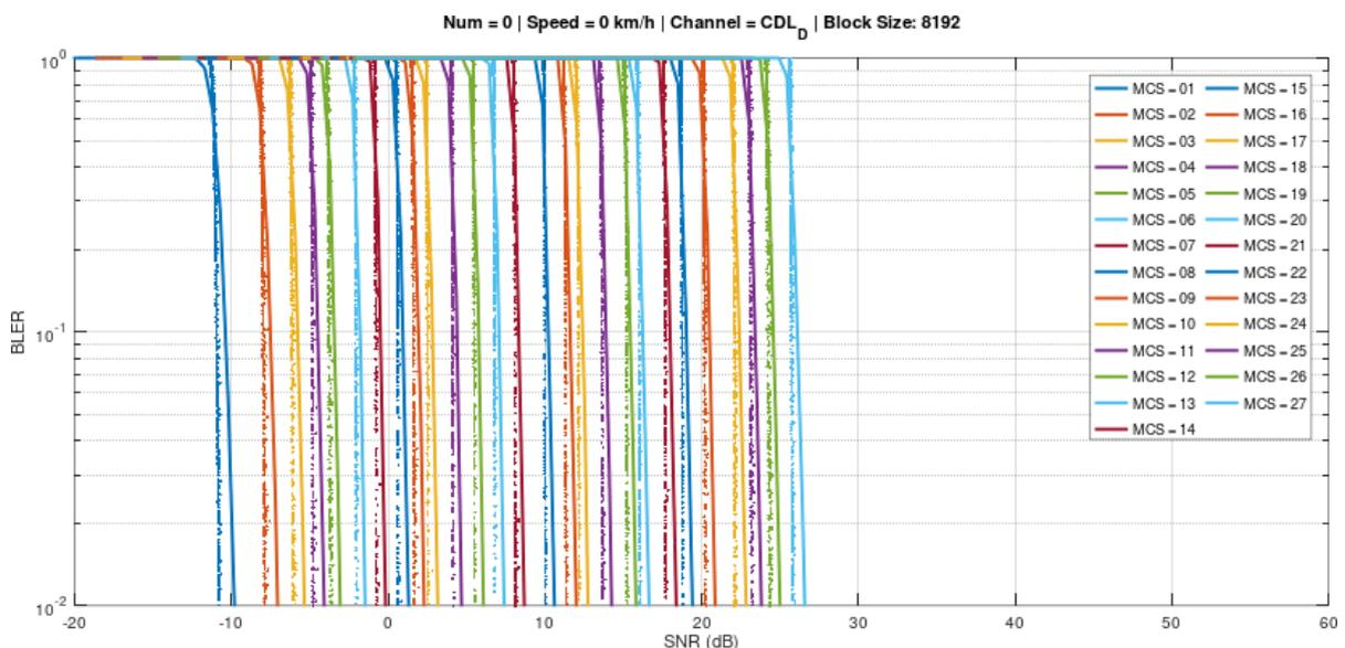
**Figure 18. BLER for the AWGN scenario and corresponding calibrated points using the EESM interface for the configuration: numerology 0, speed 0 km/h, CDL<sub>D</sub> channel model, and block size 8192.**
