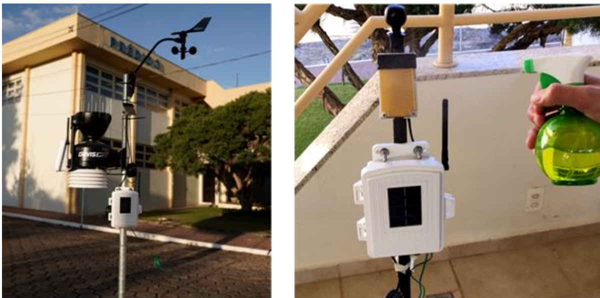
Figure 17. Weather and soil station used for the micro weather and soil monitoring applications.
