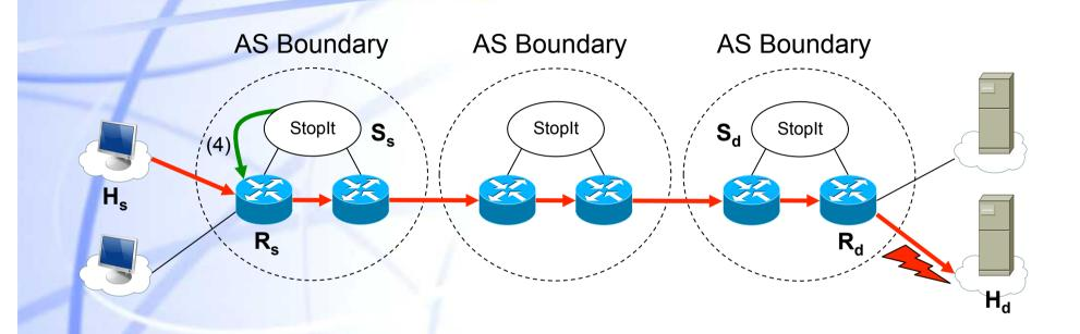
④ Ss locates Rs and sends a server-router request to the access router
