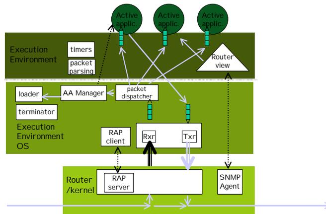
**Fig. 4.** A Router-Assistant Active Node Architecture
