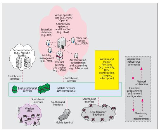
The logical centralization of SDWN offers the ability to change the forwarding of user data traffic in the access (radio and backhaul) and core transport networks, which can be used to provide functionalities such as mobility management and QoS provisioning.
