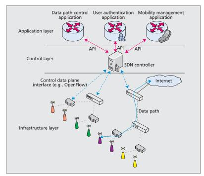
Figure 1. SDN reference architecture.
