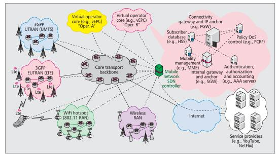
Figure 2. SDN-based mobile network architecture.
