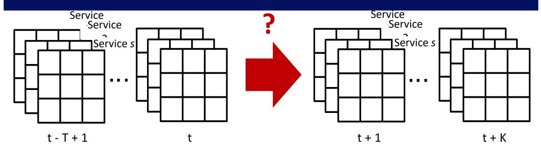
Take historical mobile traffic measurements for multiple services as input and predict future mobile traffic consumption for all services at all base stations simultaneously.
