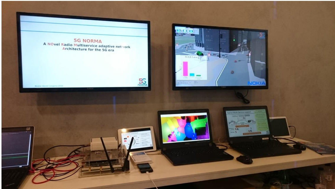
Figure 3-4. MWC'16 Setup: The software demo presented on the monitor (top right), with Simulation and GUI running on the two laptops (bottom right).
