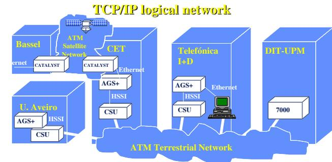
Therefore, the ATM core network supported simultaneously isochronous 2 Mbit/s traffic transporting compressed video and audio from the H.261 codecs and asynchronous IP traffic transporting compressed video and audio, plus data, from M-JPEG compression cards in the CSCW workstations.
