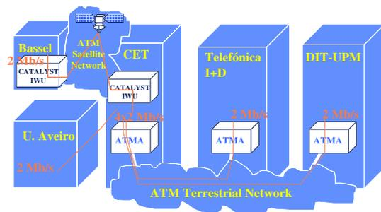
The point to point circuit network was built making advantage of the circuit emulation capabilities of ATM. ATM adapters manufactured by TID were placed at CET, TID and DIT-UPM. These ATM
