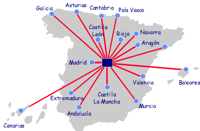
Figure 3. Topology of the RedIris IP/ATM backbone
