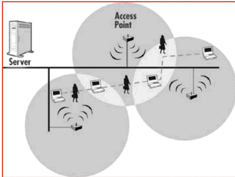
**Figure 4:** Handing off between WAN access points (courtesy <http://www.pulsewan.com>)
