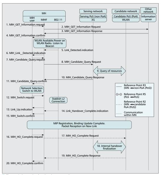
The MN should be able to discover whether the network supports IEEE 802.21 by the use of a discovery mechanism or information obtained by MIIS through another interface. It is also important that the MN is able to obtain MIIS information even before the authentication in the PoA is performed.
