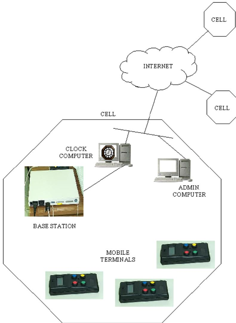
Figure 1. System architecture
