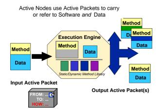
Fig. 1. An active packet traversing an active node
