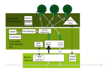
Fig. 4. A Router-Assistant Active Node Architecture
