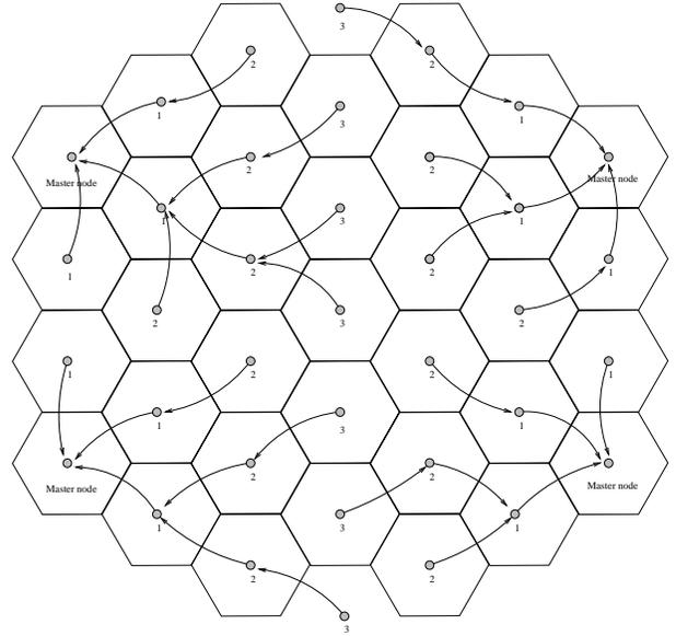
Fig. 5. Location packet routes (sample), four master nodes
