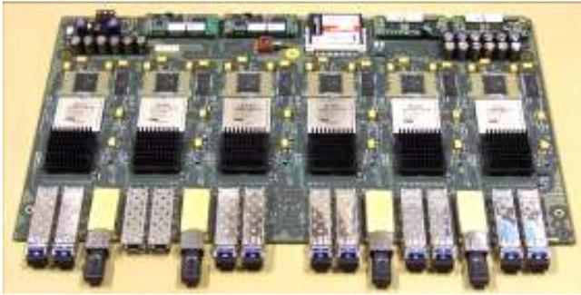
**Figure 2: AsPON Access Multiplexer blade**
